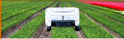
A field robot moves through a tulip field in Woldendorp, using cameras with AI image recognition to scan the plants and identify and treat diseased tulips. These autonomous robots demonstrate agricultural technologies designed for the future of crop management.
